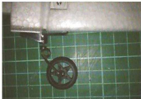
Tail wheel fixed before fitting rudder in place
