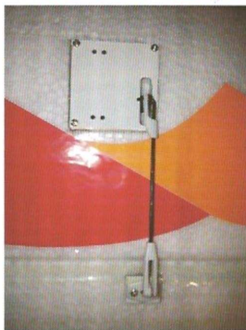
Aileron servo connected, included tape reinforces hinge line
