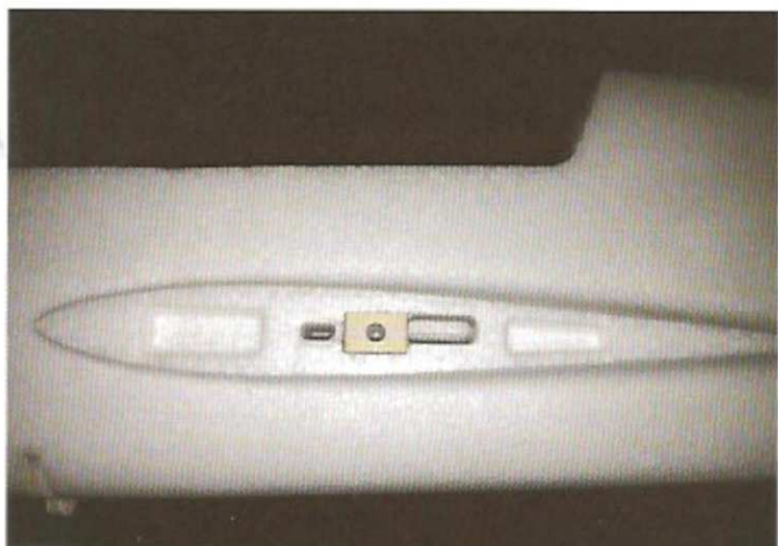
Moulded-in wing root reinforced for carbon spar and recessed for lugs of wing panels
