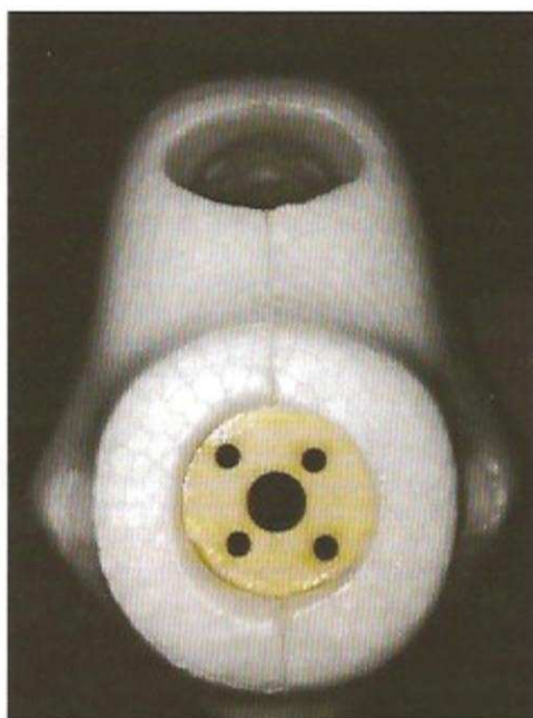
Head on view of motor mounting ring, pre-drilled to suit recommended motor
