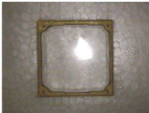
Ply servo cover frames are pre-drilled
