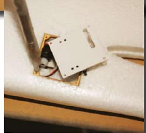
Ease out the holes in ply mounting plate before running self tappers through
