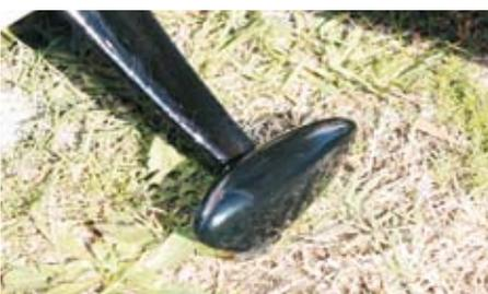
Fairing taped to uc wire and cyanoed at fuselage end
