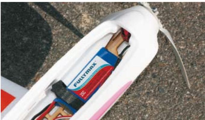
Fullymax fully forward. CofG is slightly aft with recommended 1,800 mAh. Flew much better with heavier 2,200 3S. High power to weight ratio hauled it vertically from take off and it kept going up
