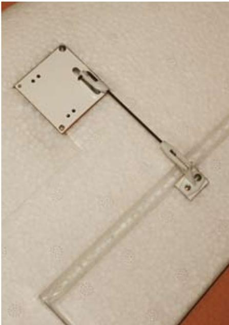
Servo linkage with keeper at one end and kwiklink the other (yes two screws left to fit)
