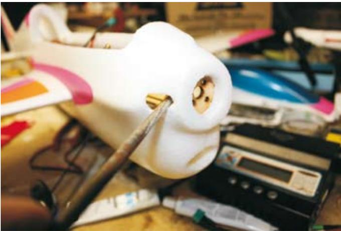
Filing the plywood motor mount is required if using the upgraded motor otherwise wires foul outer casing
